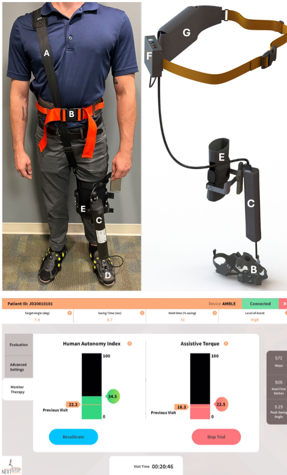
Fig. 1 (Top) AMBLE device and its key sub-systems [12]. A Shoulder strap, B gait belt, C actuator unit, D sensor crampon, E knee brace, F control box, G battery (not shown). (Bottom) User app showing a snapshot of real-time outcomes and therapy inputs (top panel widgets)
